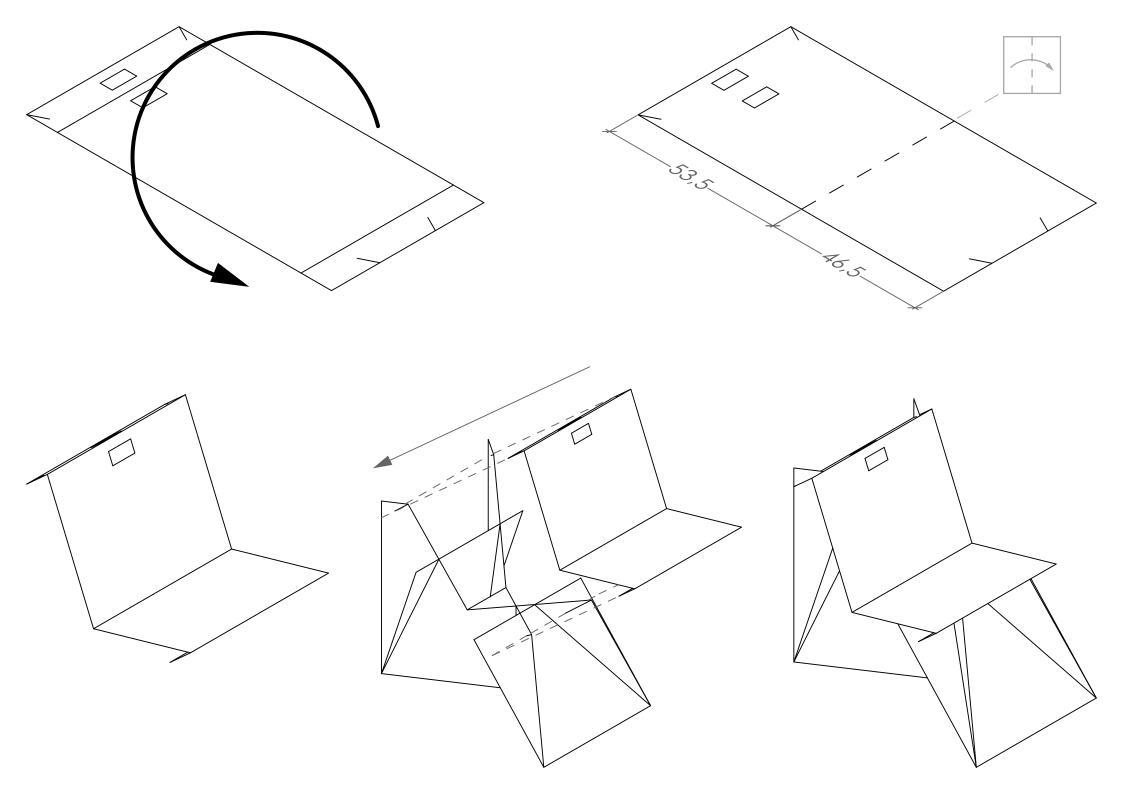
This project was made using only one 100x170cm sheet of cardboard, reducing the waste to a minimum. The chair can be dissassembled and easily transported. The construction manual and the 3d file will be released as open source so it can be build and developed further by others to hopefully achieve the stability I wanted to reach for in the beginning.
