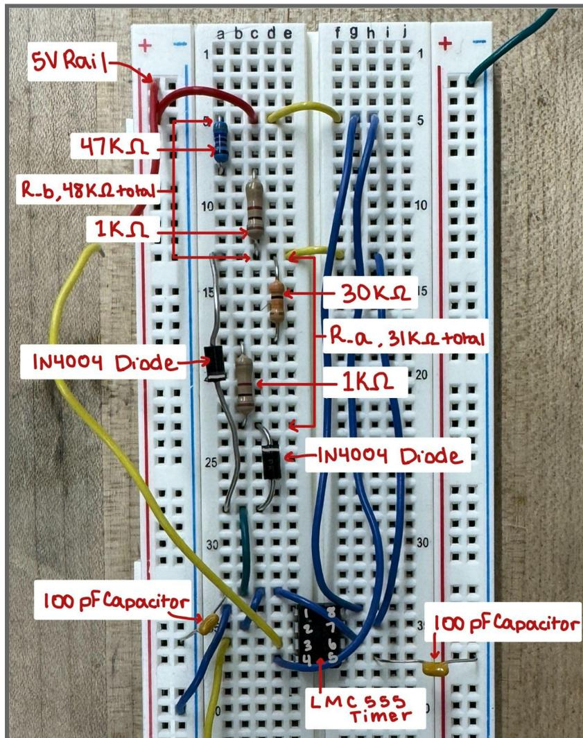
Figure 3. 555 Timer Breadboard Circuit
