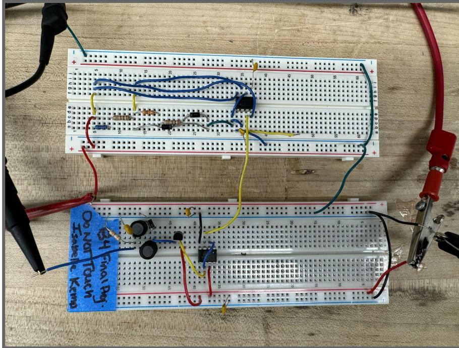
Figure 2. *Final Breadboard Setup of Buck Converter Circuit*
