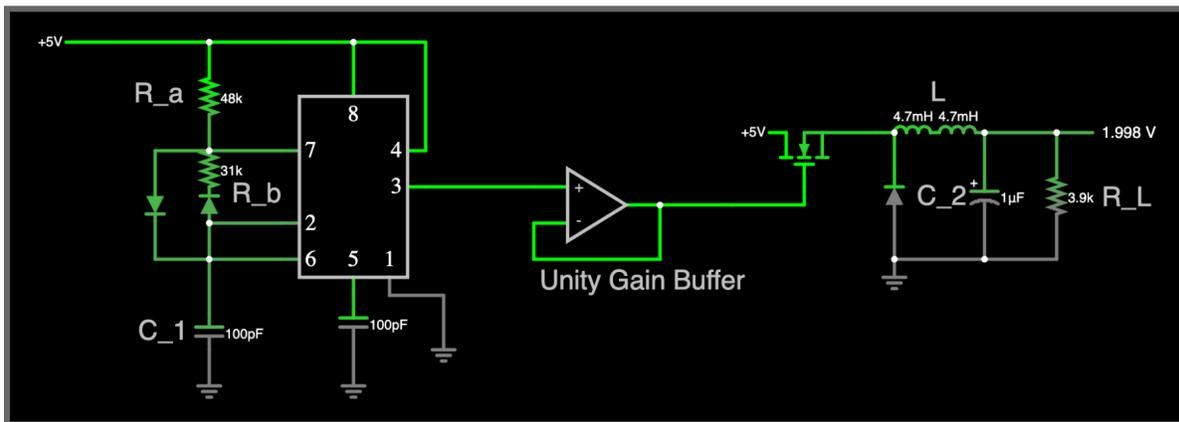
Figure 1. Falstad Simulation of 555 Timer supplying a Square Wave to the Buck Converter
