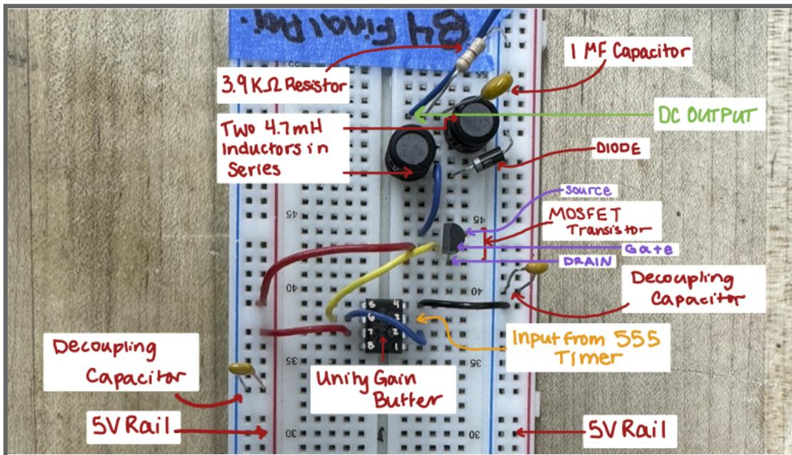
Figure 4. *Unity Gain Buffer and Buck Converter Breadboard Circuits*
