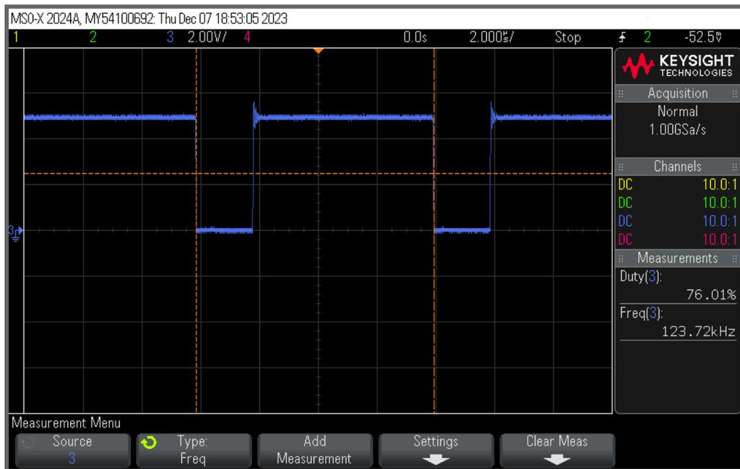
Figure 6. Output Square Wave of 555 Timer and Input of Unity Gain Buffer
