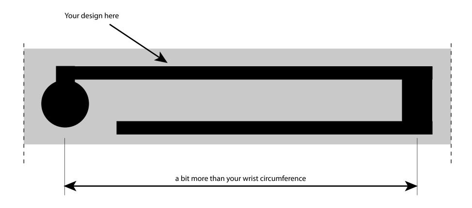
The black shape is needed to provide space for the battery, copper traces and magnet. The remaining space is up to you to fill in.
