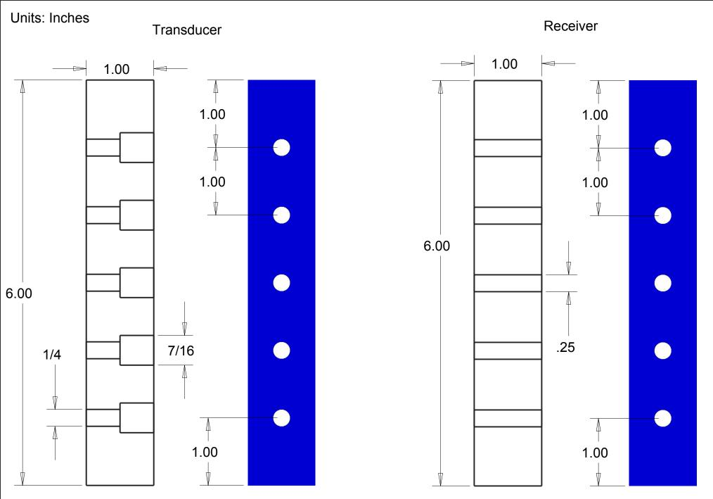
To make the 1/4 in acylic rods fit into the 1/4 in diamenter holes take an acylic rod and break a corner off at a end. Twist and insert to a depth of approximently .4 in into the wax
