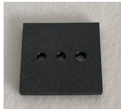
A 15: 2x Graphitelektrode (50x50x5mm)
