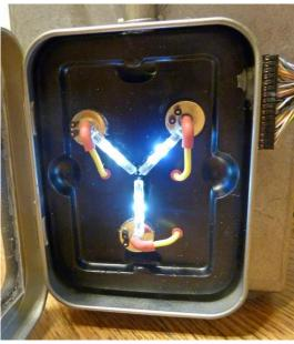
The "vacuum tubes" started out as real vacuum tubes. Wrap the tubes in a paper towel then gently break the glass. It doesn't take much. Using the insides, an LED will fit up inside. The bases are those LED tea lights from the dollar store, painted black. The "glass" parts are cut down plastic candy tubes from eBay.
