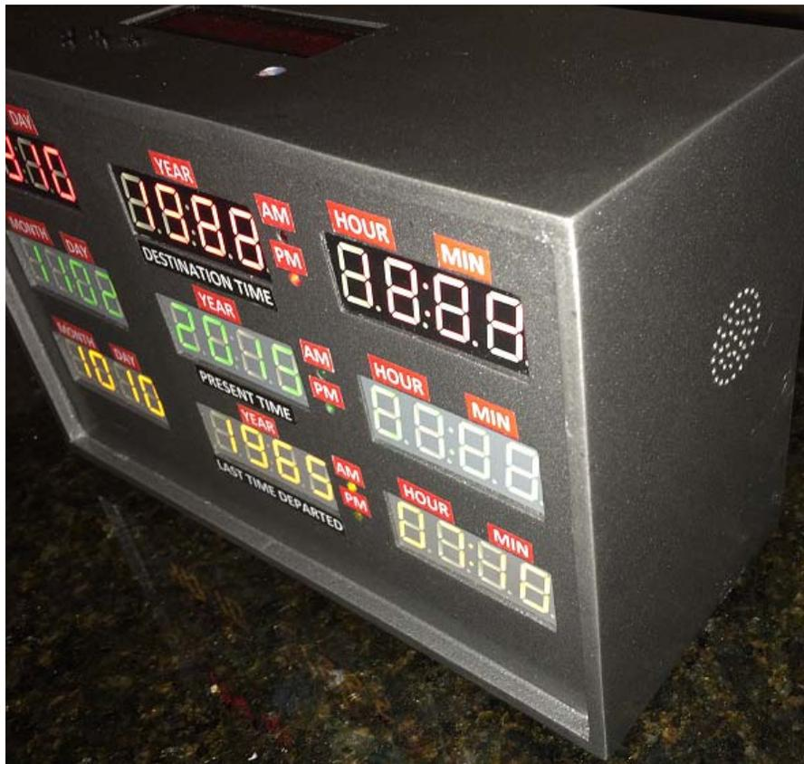
When the clock first powers on, a power on message is also announced after 5 seconds.
