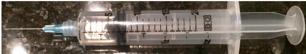
Figure 5.12 – Cement Applicator Syringe
