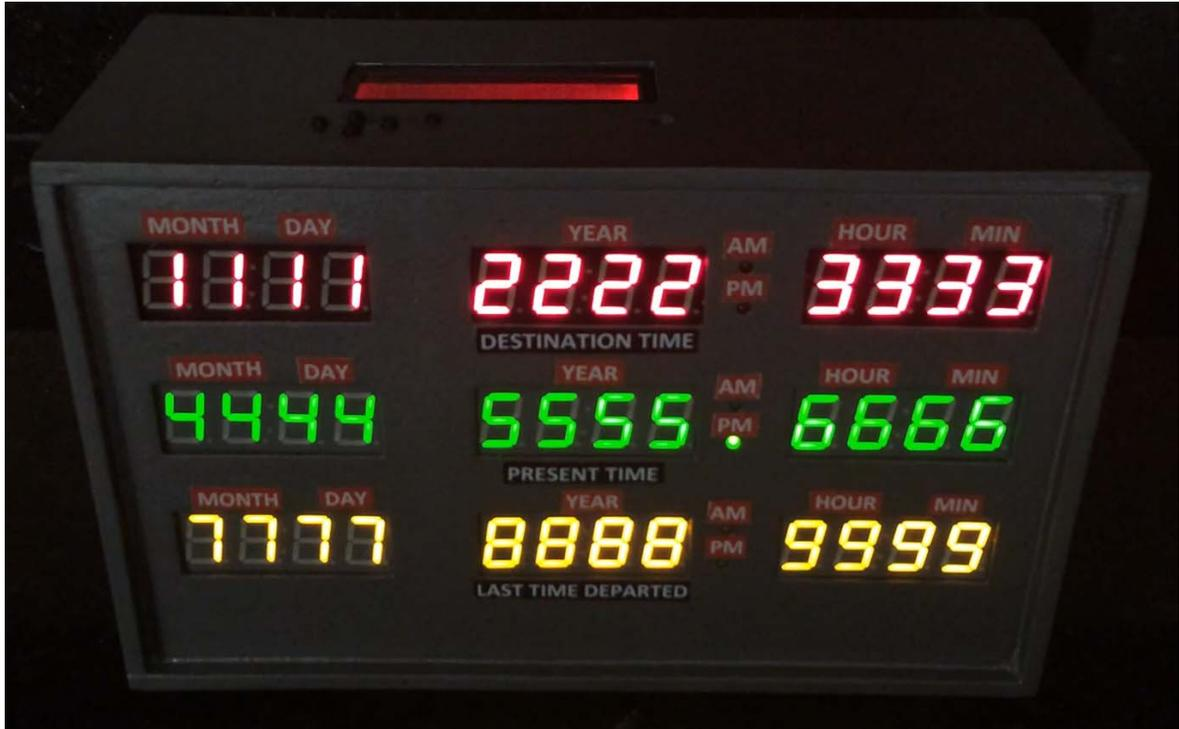
A few seconds after the numbers appear, a power on message can be heard. At this point each display will begin updating. The update occurs based on the actual real time clock seconds value so it may take 30 seconds before all the displays have been updated initially.
