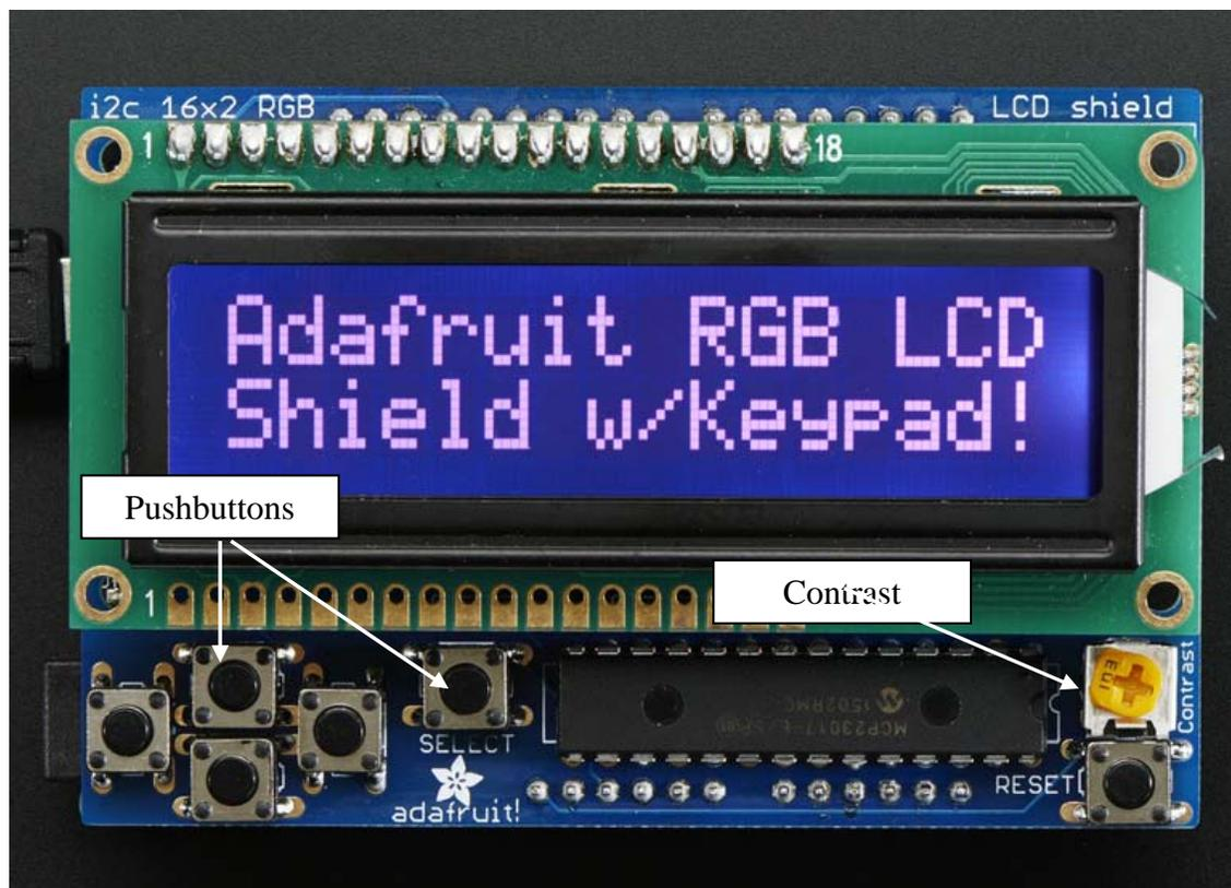
Figure 2.81 – RGB LCD Shield
