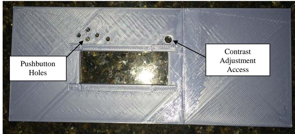
Figure 5.91 – LED Front Inside View
