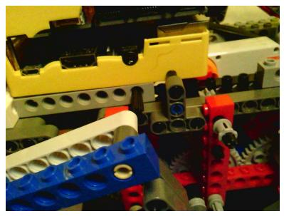
Note the upside-down "T". There will be a red bracket holding the BrickPi in place. The blue pin on the other side(image below) has to be directly opposite the "T" bracket.
