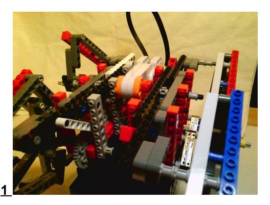
You must raise the surface of the torso so that the BrickPi can sit without interference by the motor. Note how the 2 rear 15 axles hold the wires down and the middle one goes through the motor.
