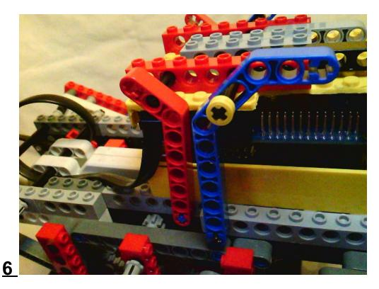
Both sides look the same, except that the red bent beam on the right side is connected by the blue axle/connector peg while on the left side the red bent beam is connected by the above "T".
