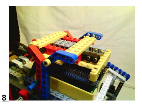
Put a 2-2x8 flat plate between the bent beams to help stabilize the BrickPi.
