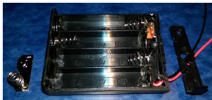
Figure 2: Plastic retainer (on the right side) and the lower rear contact have been removed. The switch can be seen attached to the holder on the upper right.
