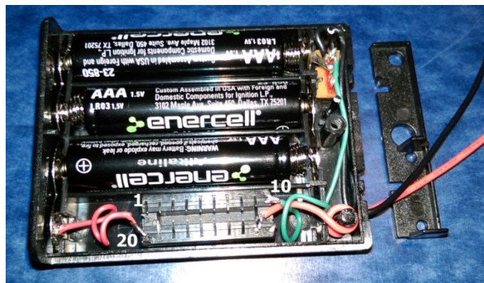
Figure 4: The original red wire is soldered to IC Pin 12 (lower right). One end of a wire is soldered to the lower left contact and the other end to MCU Pin 20. Another wire has one end soldered to IC Pin 10 and its other end to a terminal on the switch (which also has a black wire). Note that Pin 1 is near a small notch at the end of the socket.
