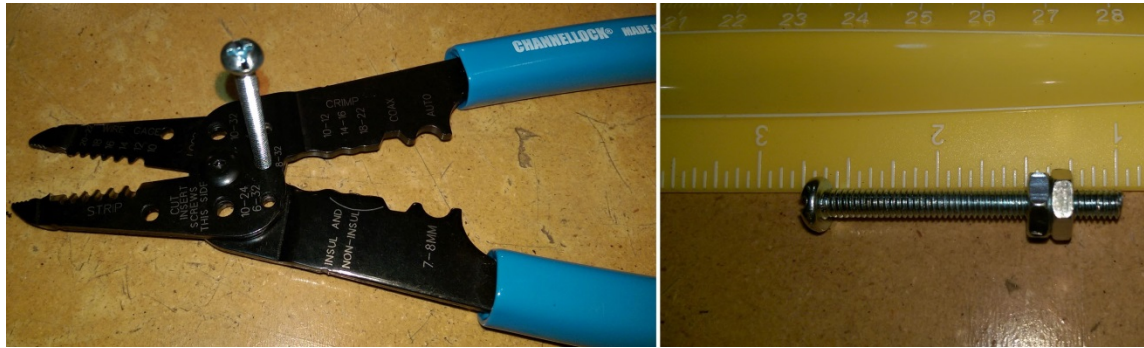
Figure 6: Left: The 8-32 screw positioned into the screw cutter. Right: Two nuts have been added to the screw to help stabilize the screw once installed.
