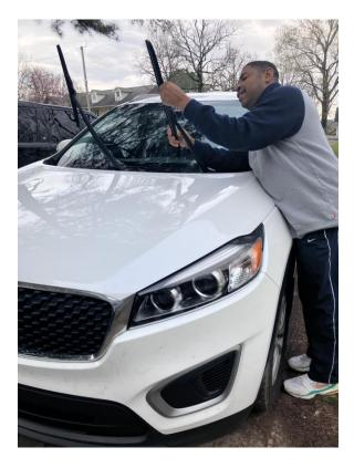
Pull the blade straight down toward the windshield to remove old blade
