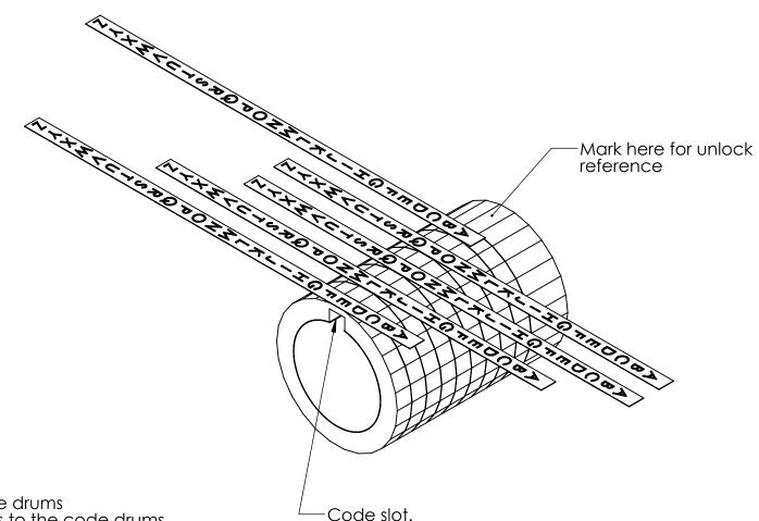
The freely rotating parts are the code drums You will ned to attach the letter strips to the code drums
