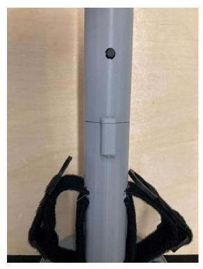
11. Press the connecting Case into the Motor and Battery Housing, lining up the screw holes and ensuring that the power button is on the opposite side as the finger contour grip.
