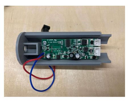
6. Fasten the PCB to the PCB and Power Jack Casing with the two PCB Mounting Screws set aside earlier.
