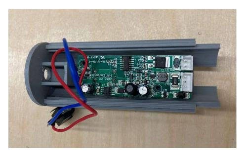
5. Align the PCB with the two mounting holes in the PCB and Power Jack Casing. The push button should fit through the hole behind.
