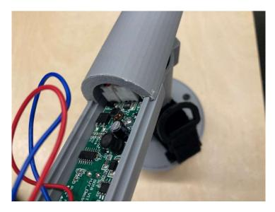
10. Align the slots of the Casing Cover and the PCB and Power Jack Casing. Slide the Casing up around the PCB, carefully bending the wires if necessary.
