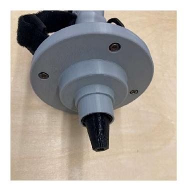
14. Press the Snapfit Opening to Hex Bit Adapter onto the Scrubber end of the device.
