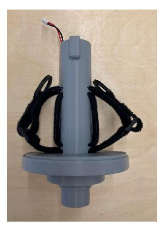
3. Carefully push the Motor and Battery Housing down over the motor.
