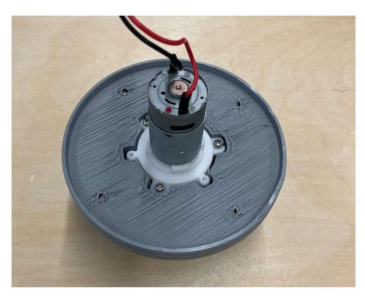
1. Place the Motor and Gearbox into the Gearbox Housing. Fasten the Gearbox to the Gearbox Housing with the three of the Motor End Screws set aside earlier.
