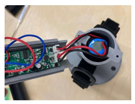
9. Connect the wires from the battery and motor into their respective connectors on the PCB.
