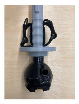
3. Use duct tape or glue to secure the Vacuum Shroud to the Gearbox Housing to prevent rotation. Glue will have a better connection, but duct tape will allow easier removal in the future.
