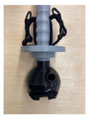
2. Rotate the Vacuum Shroud so that its opening is on the same side as the finger grip.
