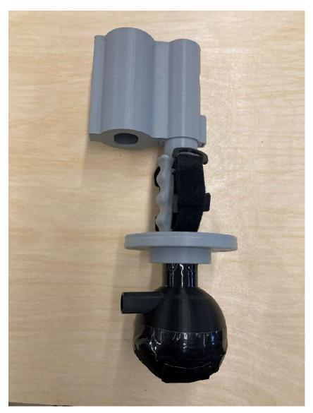
5. If you are building the **scrubber for the recommended Brigii vacuum**, slide the Brigii Vacuum Holder onto the device so that the power button shows through the hole and the slot for the vacuum sits above the finger contour grip.
