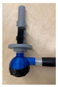
4. If you are building the **setup that works with any vacuum**, insert your 3D printed adapter from Step 4 into the opening in the Vacuum Shroud. Then, insert your vacuum hose. Your Wheelchair Tire Scrubber is complete!
