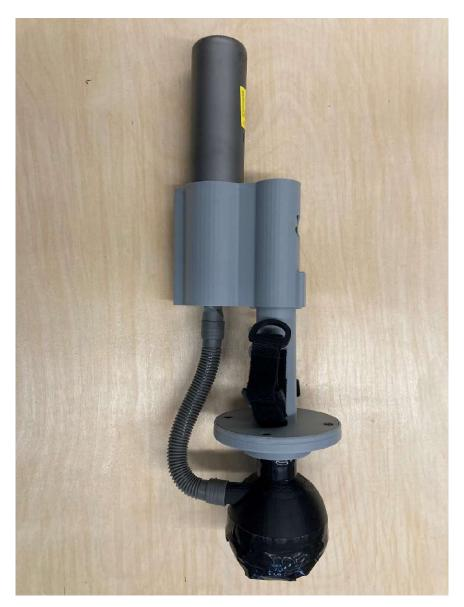
7. Connect the Brigii Vacuum Hose so that the wide end connects to the Brigii Vacuum through the bottom of the Brigii Vacuum Holder and the round end connects to the Brigii Vacuum Shroud. Adding duct tape around the shroud connection improves suction. Your Wheelchair Tire Scrubber is complete!
