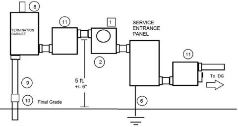
All DG equipment must be permanently labeled according to NEC 705.10. Alliant Energy requires self-sticking brass or rigid plastic permanent label at meter socket for multiple or net metering.
