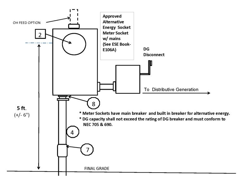
All DG equipment must be permanently labeled according to NEC 705.10.
