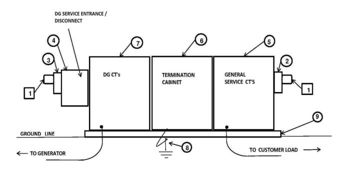
All DG equipment must be permanently labeled according to NEC 705.10.
