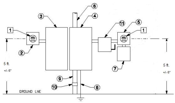
524A. NET-METERED SELF-CONTAINED WHERE SERVICE PLUS DISTRIBUTED GENERATION DOES NOT EXCEED 120% OF SERVICE PANEL BUSS CAPACITY
