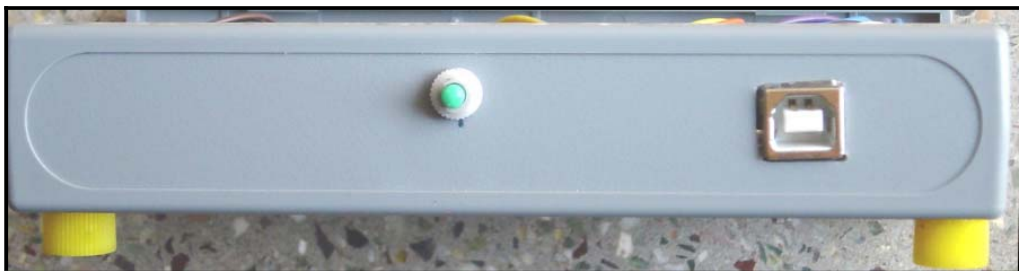
Figure 10, Rear panel showing USB connector and Reset switch
