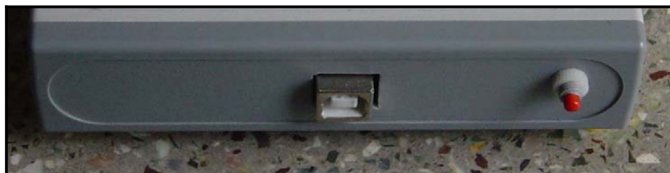
Figure 5, Rear panel showing USB connector and Reset switch
