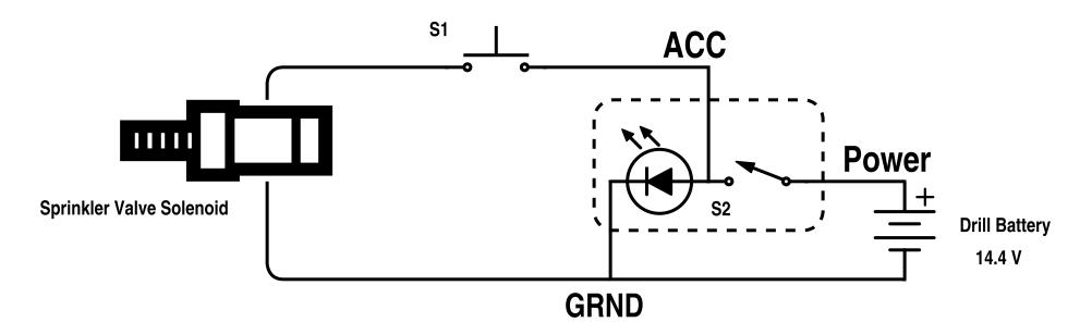
S2 is a LED embedded automotive switch with a spring loaded cover that acts as a system "Safe/Arm" S1 is a large momentary push-button for "Launch" or "Fire" The sprinkler valve typically works at 24 VDC but for this purpose, 14.4 works fine The labels shown are pins off the S2 switch
