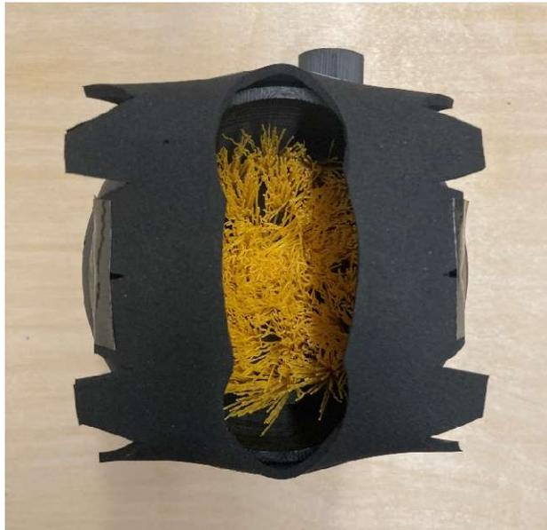
10. Use small pieces of duct tape to tape down the center two flaps on each of the long sides of the foam cutout. Make sure there is a 1-inch gap between them.
