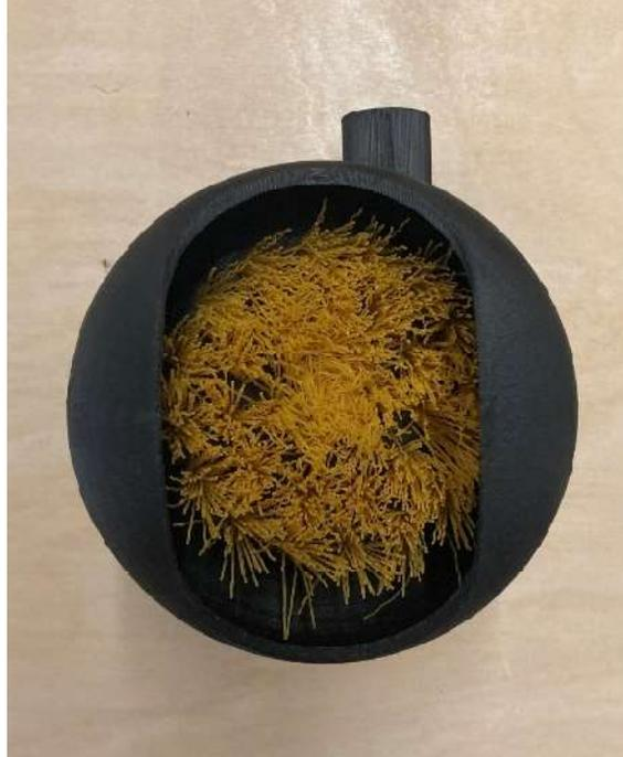
7. Insert the Bristle Attachment from Step 2 into the Vacuum Shroud that you printed. The end of the Bristles should point to the large tire opening.
