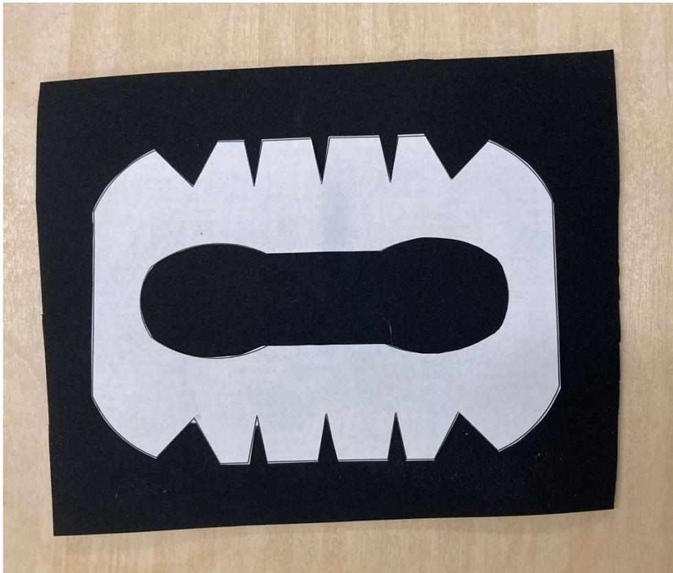
4. Cut a piece of foam slightly larger than the guide and adhere the guide to the foam.
