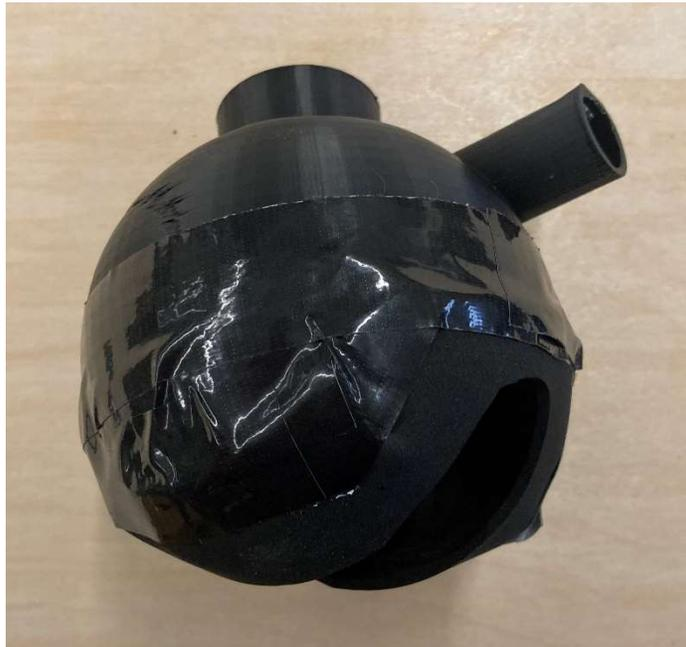
12. Use longer pieces of duct tape around the outer edge to ensure a secure connection and a vacuum seal.
