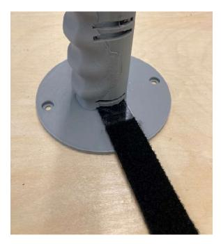
8. Slide the hook (hard) end of the strap through the bottom strap slot in the Motor and Battery Housing with the adhesive backing facing up.
