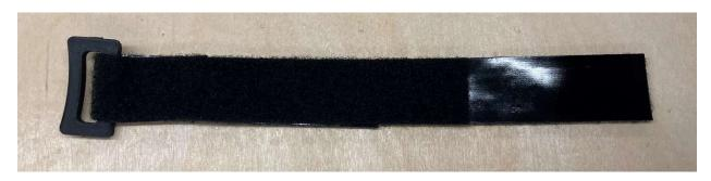
4. Remove the adhesive backing from the remaining strip. Cut a 4 inch piece of the loop (soft) Velcro. Remove its adhesive backing and attach to the longer strip starting at the end with the clip. There should be about 2-3 inches of exposed adhesive at the bottom.
