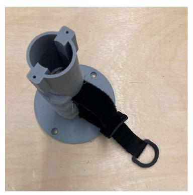
15. Peel off the adhesive backing on the end of the strap. Guide the strap through Strap Clip 1 and have the straight edge of the Strap Clip touch the adhesive at its midpoint. Fold the adhesive over around Strap Clip 1 and adhere the two sides of the strap together, leaving no exposed adhesive.
