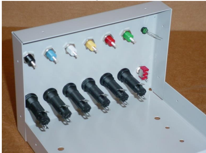
Install all binding posts, fuse holders and switch hot glue LED holder and LED in place
