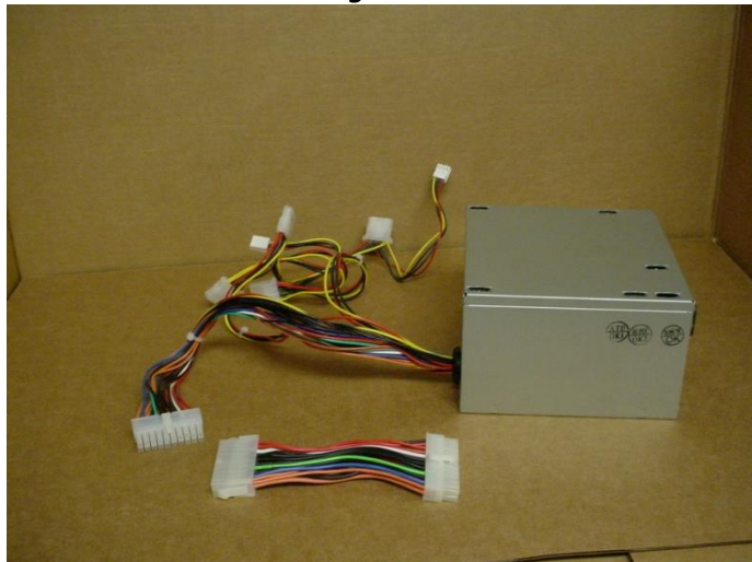
Purchase/Harvest ATX power supply and 20 pin ATX power supply extension (NOTE: The wire colors do not always match)
