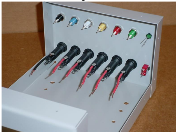
Solder wires to the fuse holders
