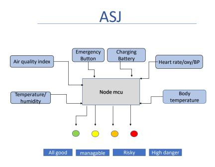
This Jacket give indication to worker they are working in good safe environment or not. Jacket also sense health data and send to monitoring base if worker press the Emergency Button.
