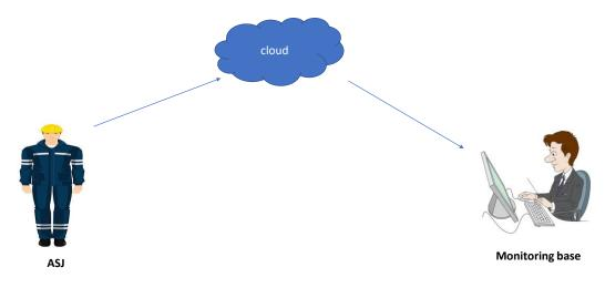
ASJ indicate data to monitoring base when worker press the emergency button, and ASJ also indicate the type of zone where worker are working .
