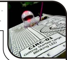
grab the parts listed below, pin the layout sheet to your breadboard and then plug everything in. Once the circuit is assembled you'll need to upload the program. To do this plug the Arduino board into your USB port. Then select the proper port in Tools > Serial Port > (the comm port of your Arduino). Next upload the program by going to File > Upload to I/O Board (ctrl+U). Finally bask in the glory and possibility that controlling lights offers.
