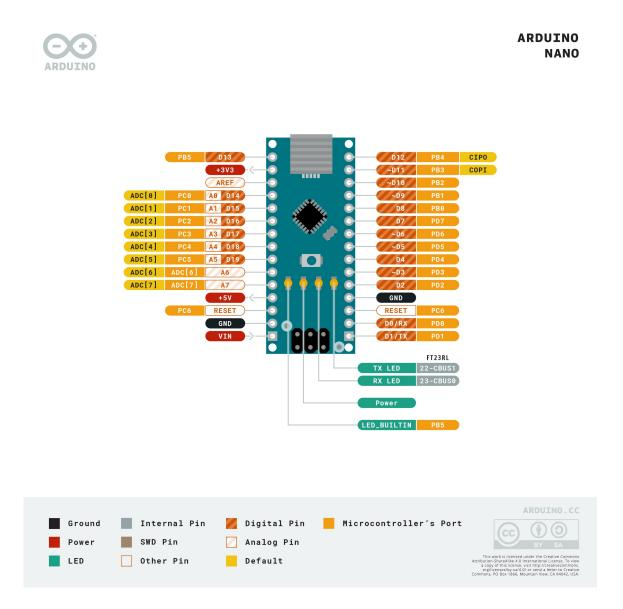
The Arduino Nano is equipped with a variety of pins and features that enable users to interact with and control various electronic components. These pins are divided into three main categories:
