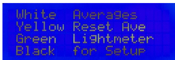
LCD splash screen, due to size limitation only subset of info can be displayed.
