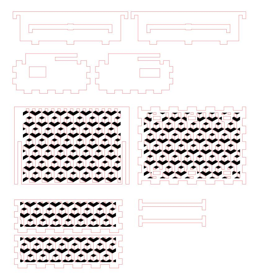
If you want the box without the cradle for the circuit board, substitute the parts on the left matching these parts below.
