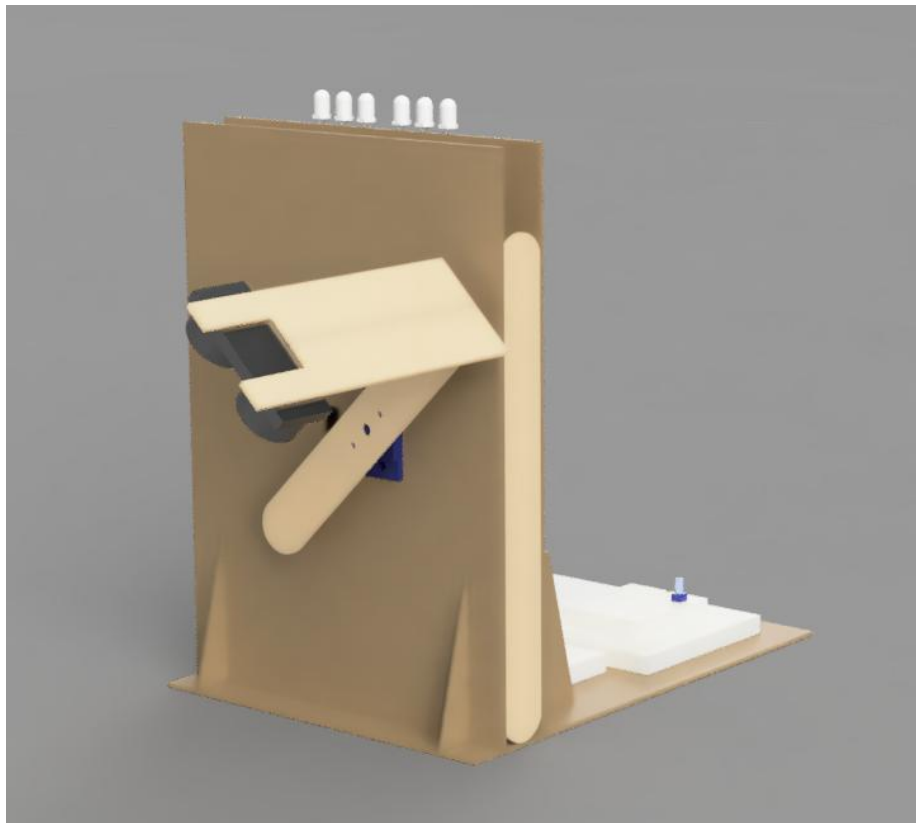
Figure A6. Full assembly with ultrasonic sensor, potentiometer, actuator, LEDs, and arduino & breadboard place markers.
