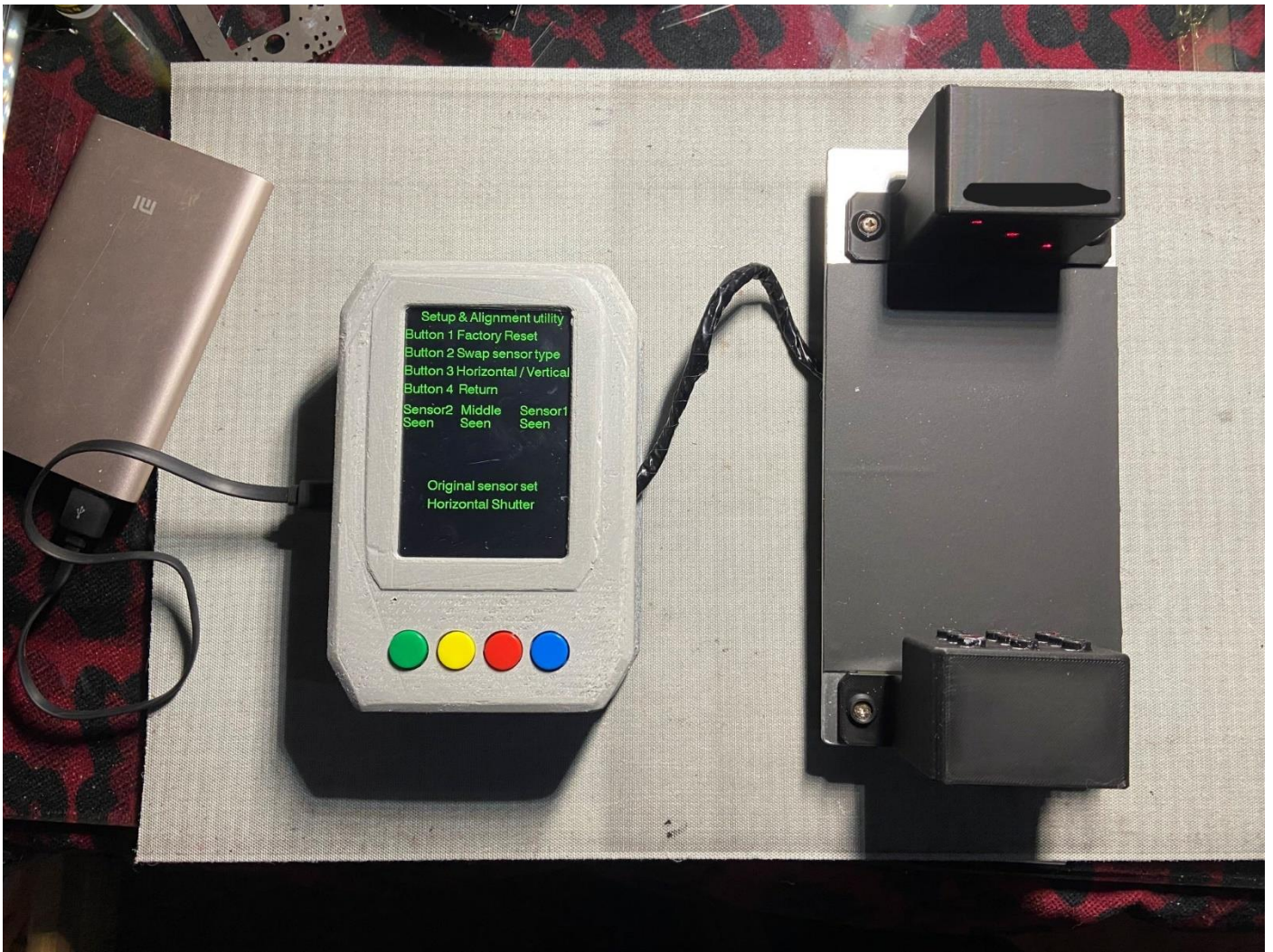
3d printed version. Note lasers & sensors are arranged diagonally, 32mm spacing horizontally & 20mm vertically. This way the same sensor frame can be used for horizontal or vertical shutters. It does however make it a little more tricky to line up the film-gate with the Lasers.
