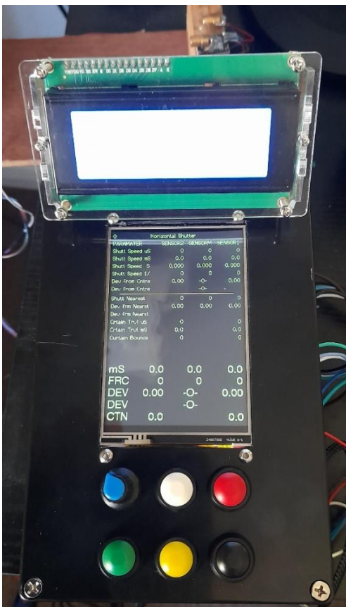
Here is the ESP32 Shutter Tester in a larger 200-120-75 project box, with both TFT & LCD. The LCD is mounted in an acrylic frame and bolted to the top of the project box.
