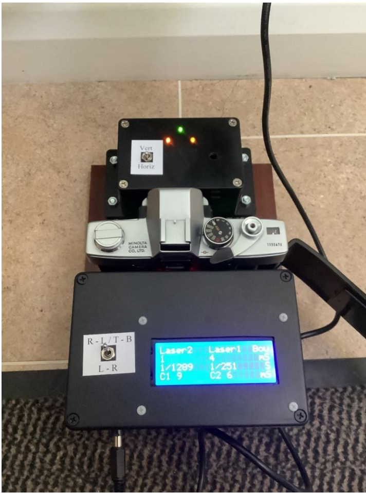
Horizontal or vertical shutters. Switch toggles horizontal or vertical Lasers.
