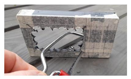
Turn the box over & using the saw marks as a reference, again score the inside of the box.
