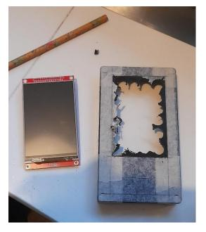
Using a junior hacksaw, or just a hacksaw blade, cut diagonally into the four corners, keeping the blade at 90 degrees
