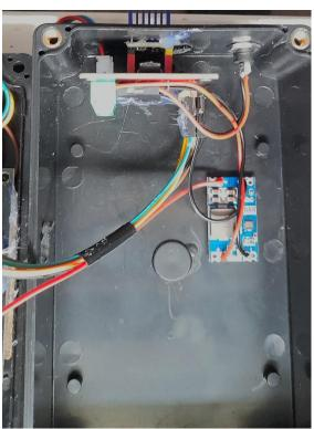
Stepper board hot-glued in position. M3 bolts will be used on the lower fixing holes for permanent mounting. Note it really is a tight squeeze to fit the stepper motor into this size project box, but it can be done. An alternate is to use the next size project box (see link in parts list document).
