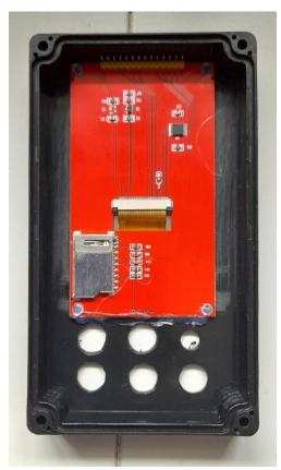
Drill the holes for the encoder (6mm) and the buttons (12mm) using a brad point drill bit. Note the bottom line of button holes should be drilled a few mm lower than shown here, to give a little more separation.
