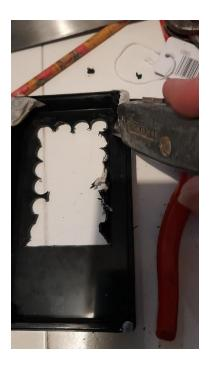
Using slip-joint pliers (as they fit into the opening) grip the lid at the score line and gently bend inwards. Do this all along the score line and repeat, each time bending a little more. Alternate this with scoring, which will get easier as the plastic bends. Eventually the plastic will snap away.
