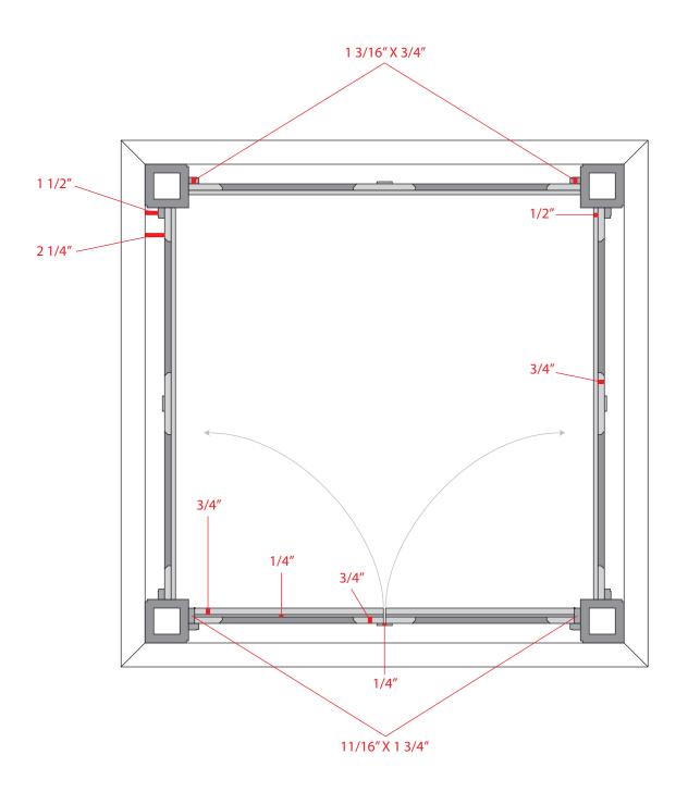
Doors are constructed with sandwiched 3/4" ply for the backing, 1/4" ply for the panels, and 3/4" for rails and stiles. Walls are constructed with 1/2" ply for the backing/panels and 3/4" for rails and stiles.
