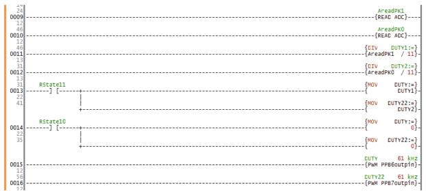
On State10 every output must be reset and all the states of the slave machines too.
