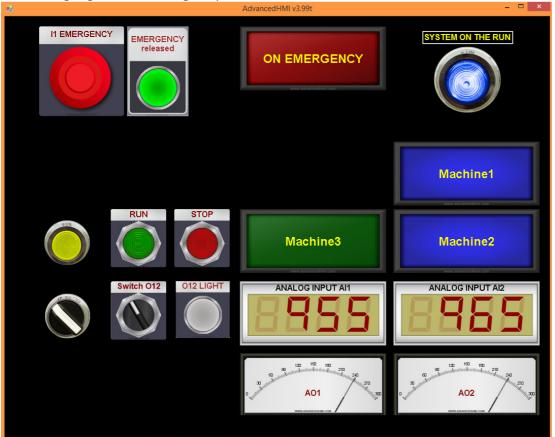
When you push the emergency: the master machine stays in state 10 (Reset of all the system) but it's not safe because at the same time the power must be switch off on the actuator (EMERGENCY RULE) and it's only done with the real mushroom push-button.
