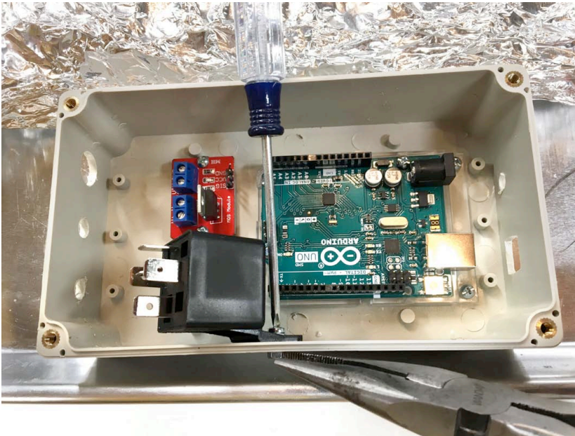
Fig. 3.2.6 - Mounting automotive relay. Wires removed for clarity of picture.
