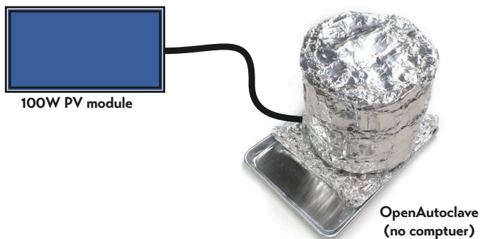
Figure 5.11b - Solar power operation with no charge controller and no computer.
