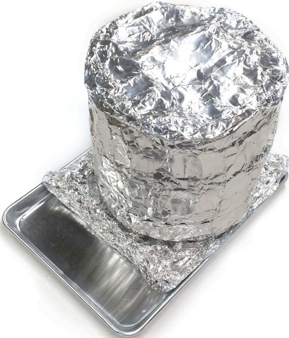
Fig. 2.0 - Insulated oven made from a stock pot, a cookie sheet, ceramic fiber insulation, foil, and foil tape
