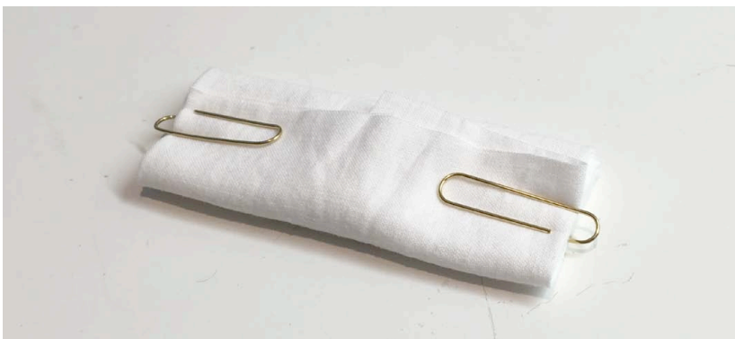
Fig. 5.3d - Biological indicator test strip shown wrapped in linen for autoclave exposure. Wrapping simulates the exposure conditions of linen-wrapped medical instruments.
