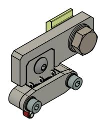
Except the limitswitch itself and the screws, the components are all 3d printed.
