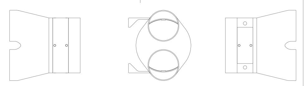
Consisting of 3 printed parts, this connector combines the two channels for ventilation to one. We use a quite strong ventilation for really getting all the fumes. From one side there are the two channels connected and from the other side a 150 mm tube.
