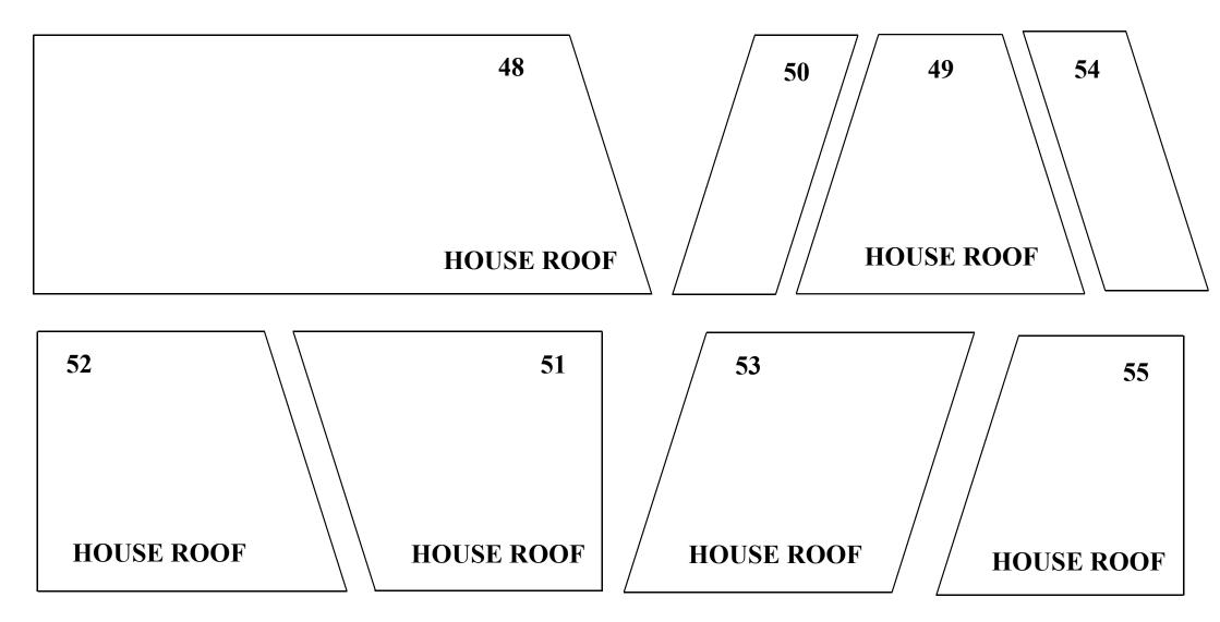
NB. Some edges of these roof parts will need bevelling where necessary to fit together
