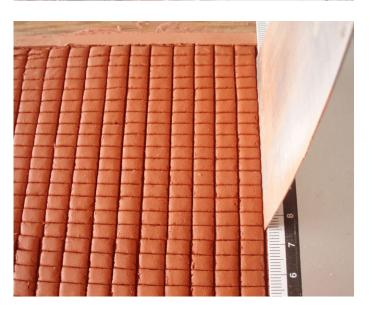
After making the horizontal cutting I proceed with the vertical ones, in stripes of 0,30/0,40 inch, depending on my needs. Before the material is totally dry I apply a light pressure on the surface to limit the smoothness caused by the slice during the cut.
