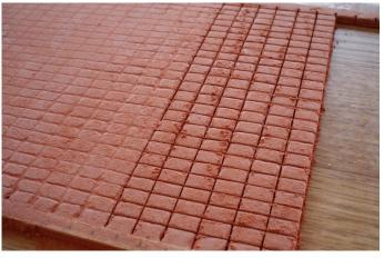
In this stage I try to separate the bricks in slices of at least 4 pieces, as you can see in the picture below. That's because the little bricks still need to be polished with a file to be finished. On a board like this you can produce more than 1300 bricks at a time, so you can see the advantage (in terms of time) to polish them in groups of 4 and not one-by-one.
